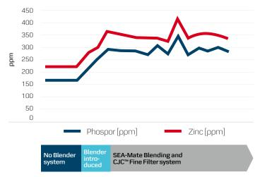
The ZDDP anti-wear additive is a crucial performance parameter for the lubrication oil by enhancing its load bearing capacity. When starting Blending-on-Board, the ZDDP additive increased almost 100% (which is similar to new system oil). By using the SEA-Mate<sup>®</sup> CJC™ Filter, high concentration of ZDDP levels are maintained due to oil refreshment as well as reduced friction and wear.
