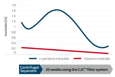
The area between the red and the blue curves represents soft particle contamination, such as resinous and oxidation degradation products as well as asphaltenes. The distinctive variation indicates an extraordinary improvement of engine crankcase system oil shortly after using the SEA-Mate® CJC™ fine filter system.
