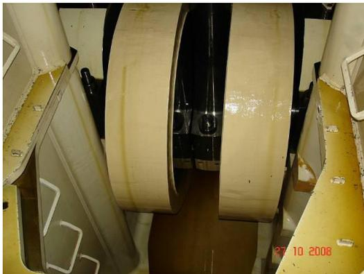
The above photograph, from a vessel that is 10 years old, shows how the replenishment system oil into the crankcase results in a significantly cleaner condition. In this particular case, the engine had only been blending onboard for three months.
