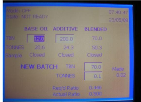
Once several blends are made, the input for the base oil BN and the additive BN will be constant, therefore, all the Chief Engineer needs to enter is the desired BN of the blend (in this case 70 BN) and the amount of cylinder oil to blend. Once this is completed, the operation is automatic and the Chief can leave the unit and perform other duties.
