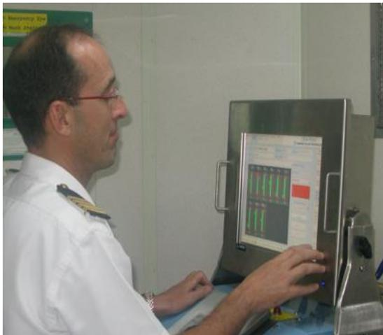
The analyzer has the capability of running a complete analysis in 6 minutes with no need to decant the sample since the measurement is taken through the capped bottle. This non-destructive sampling technique allows the vessel to retain samples for either legal purposes or for further more advanced testing.
